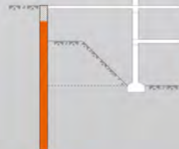
BERMA Y LOSAS ("SEMI-TOP-DOWN")
